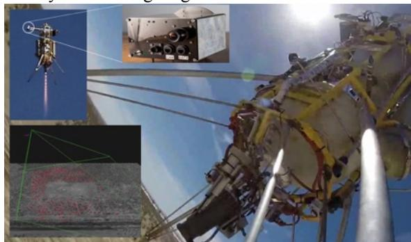
**Figure 1.** Astrobotic’s TRN field test performing precision landing and hazard avoidance in Mojave, CA.
